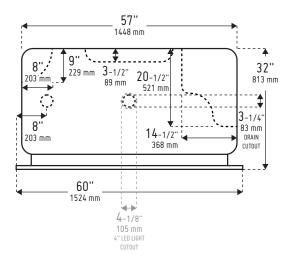
This unit is available as an End Drain or Centre Drain configuration. Both configurations are shown in the above drawing - Please specifiy Drain (LD/RD/CD) and seat configurations (LS/RS/NS) when ordering.
