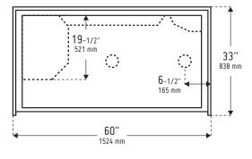
This unit is available as an End Drain or Centre Drain configuration.
